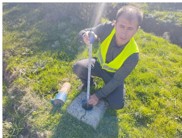
Fig. 3. Groundwater level measurement
