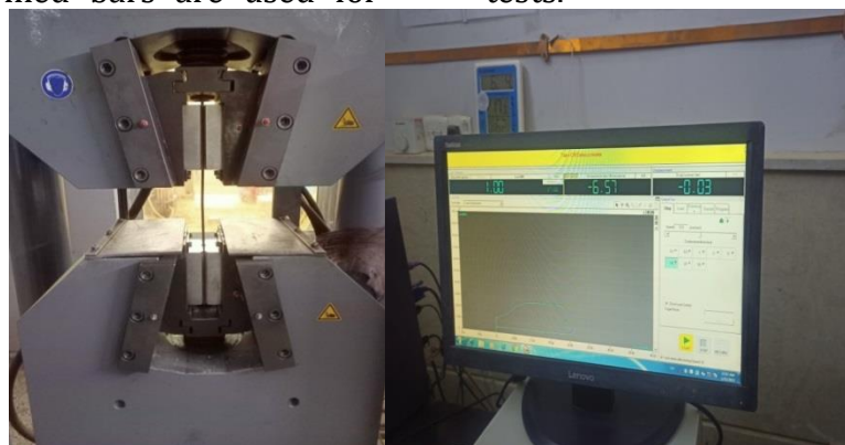
Figure 1 Test Setup for Steel Bar
