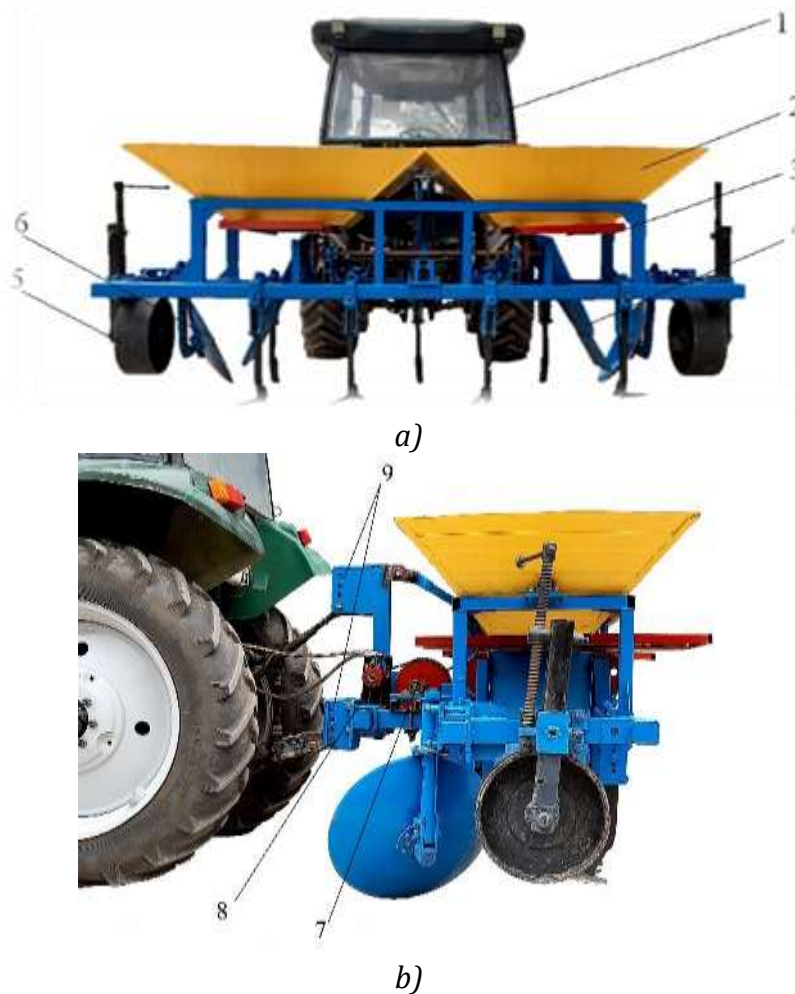
1 – tractor; 2 – fertilizer bunker; 3 – quantification device; 4 – fertilizer transfer channel; 5 – support wheel; 6 – spherical disc; 7 – transmission star; 8 – hydromotor; 9 – suspension device
